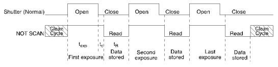
Figure 16. Free Run Timing Diagram
